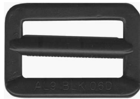
AL9-BLK knurled adjuster bar 1 3/4" x 1" forged steel, black plated 5,000 lb Commercial version of PS22040
