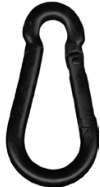
SP62-BLACK 5/16" steel wire, black 3 3/16" length 3/8" gate opening
