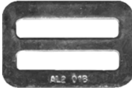
AL2 1 3/4" x 5/16" slots alloy steel, zinc plated 3,000 lb. Also available in black phosphate.
