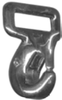
SN715 3/4" or 1" zinc die cast, nickel 1 3/4" length
