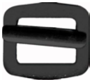
AL101-BLK channel adjuster bar 1" steel, black plated 1,000 lb. SPECIAL ORDER
