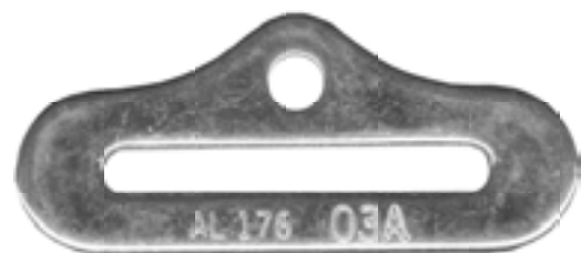
AL176 Bolt-In End Fitting 1 3/4" x 1/4" slot, 1/4" hole alloy steel, zinc plated 3,000 lb
