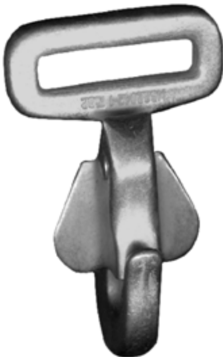
RH103 Quick Connector Snap 1 3/4" slot forged steel, cadmium plated 2,500 lb. proof load Certifies to PS22042-1 SPECIAL ORDER
