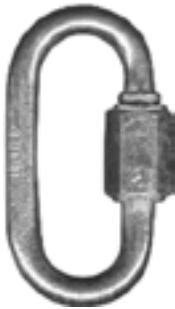
QL50 5/32" steel wire, zinc 1 9/16" length 3/16" gate opening
