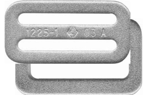
RH1224 Link & RH1225 Adapter Double Pass Buckle 1 3/4" x 3/16" slots alloy steel, cadmium plated 2,500 lb. proof load Other Double Pass Buckles Available.
