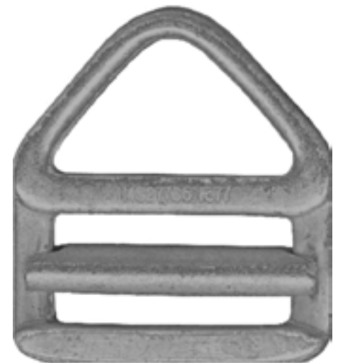
RH18 "Quick Fit Adjuster" 1 3/4" slot forged steel, cadmium plated 2,500 lb. proof load Certifies to PS27765
