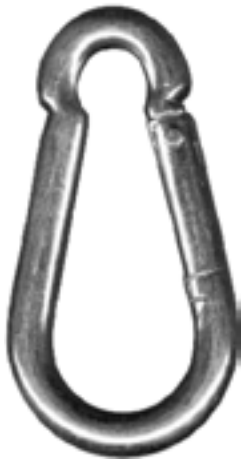
SPC63 1/4" steel wire, zinc 2 3/8" length 5/16" gate opening
