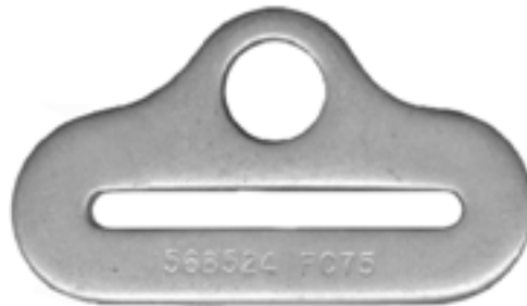
PS171 Bolt-In End Fitting 1 3/4" slot, 1/2" hole steel, cadmium plated Surplus version of 56B524
