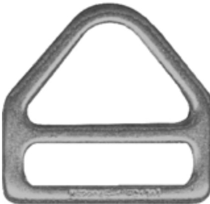
RH45 1 3/4" x 3/8" slot forged steel, cadmium plated 2,500 lb. proof load Certifies to PS22045
