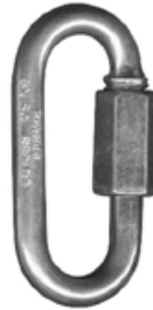
QL52 1/4" steel wire, zinc 2 1/4" length 9/32" gate opening Use QL67 for Stainless Steel
