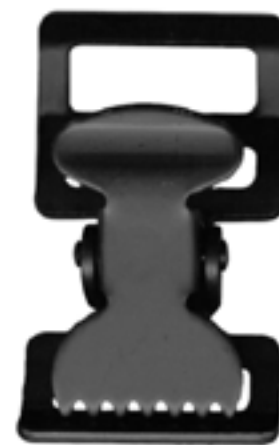
BKC6105 1" sheet steel black resin Also available to meet MS51929-2 (SPECIAL ORDER)
