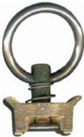
SF17 Single Stud Fitting with 1" O-Ring steel, yellow cadmium 4,000 lb. vertical breaking strength
