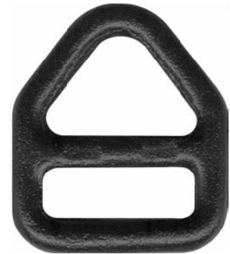
AL45/100-BLK 1" x 3/8" slot forged steel, zinc plated 4,000 lb.
