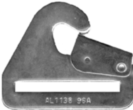
AL1138 Snap-In End Fitting 2" x 3/16" slot, 3/8" anchor point alloy steel, zinc plated 3,000 lb
