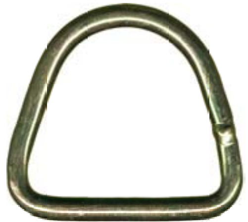
DR/200-5000 Cargo D-Ring 2" x 1 13/16" welded .250" steel wire yellow cadmium 5,000 lb.
