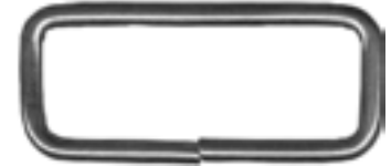
LP4950 Non-Welded Loop 1 1/2" x 1/2" .120" steel wire, nickel
