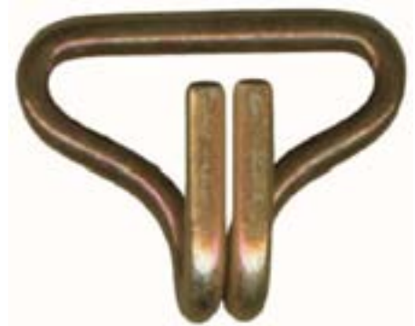
WHK-N/200-2500 Narrow Wire Hook 2" .250" steel wire, yellow cadmium 2,500 lb.
