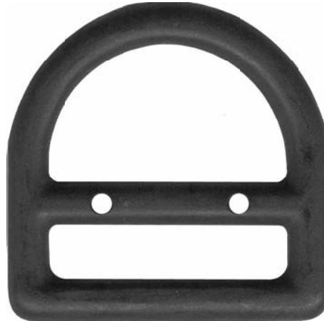
PS28-BLK Slotted D-Ring with holes in cross bar 1 3/4" x 3/8" slot forged steel, black phosphate Non-certified, surplus version of PS22046-3
