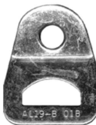
AL19-B Bolt-In End Fitting 1" x 1/2" slot, 1/2" hole 45° bend alloy steel, yellow chromate 3,000 lb
