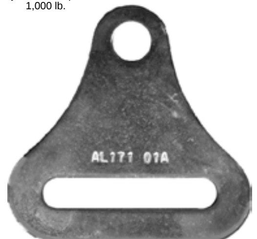
AL171 Bolt-In End Fitting 1 3/4" x 5/16" slot, 3/8" hole alloy steel, nickel plated 3,000 lb
