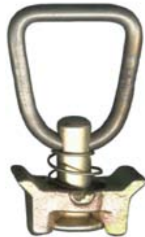
SF18/100 Single Stud Fitting with 1" D-Ring steel, yellow cadmium 4,000 lb. vertical breaking strength
