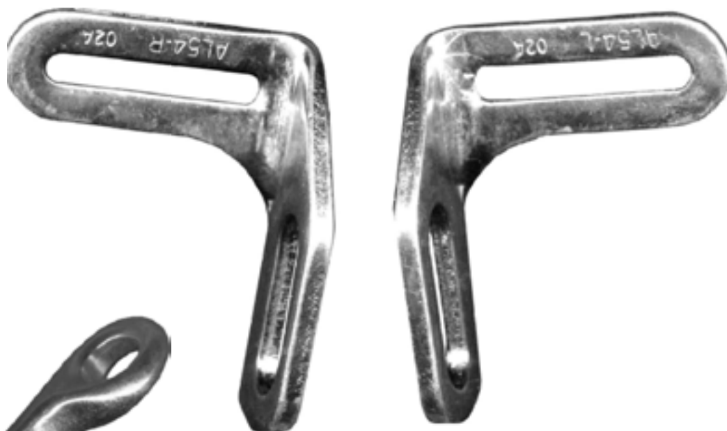
AL54-L & AL54-R Shoulder Links for Latch & Links Left & Right 1 3/4" web slot alloy steel, zinc plated 3,000 lb
