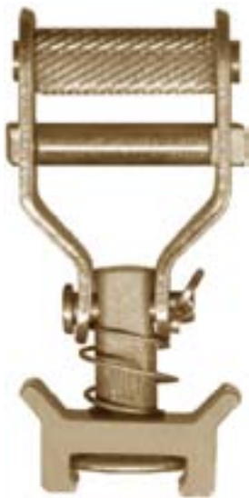
SF16 Adjustable Stud Fitting 1" steel, yellow cadmium 4,500 lb. vertical breaking strength SPECIAL ORDER
