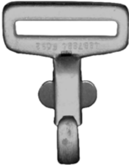
RH98 1 3/4" slot forged steel, cadmium 2,500 lb. proof load Certifies to 48B7884 SPECIAL ORDER
