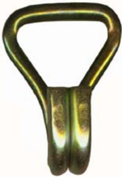
WHK-N/200-5000 Narrow Wire Hook 2" .250" steel wire, yellow cadmium 5,000 lb.
