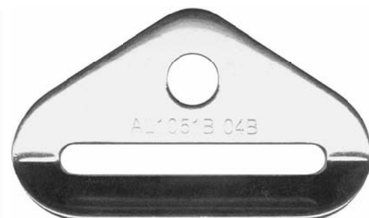
AL1051-B Bolt-In End Fitting 2" slot x 1/4", 3/8" 45° bend alloy steel, chrome 3,000 lb
