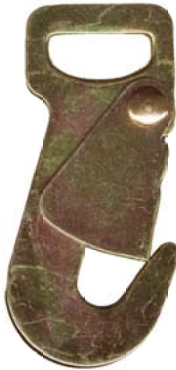
FSN/100-5000 Flat Snap Hook 1" steel, yellow cadmium 5,000 lb.
