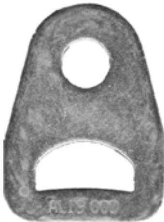
AL19 Bolt-In End Fitting 1" x 1/2" slot, 1/2" hole alloy steel, yellow chromate plated 3,000 lb
