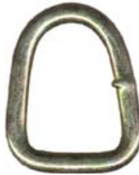
DR/100-5000 Cargo D-Ring 1" x 1 5/16" welded .250" steel wire yellow cadmium 5,000 lb.
