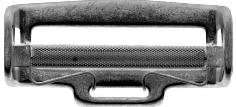
AL16-S Roller Adjuster with Spring Tensioner 3" slot alloy steel, zinc plated 3,000 lb
