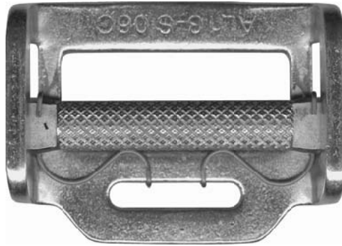
AL13-S Roller Adjuster with Spring Tensioner 1 3/4" slot alloy steel, zinc plated 2,500 lb
