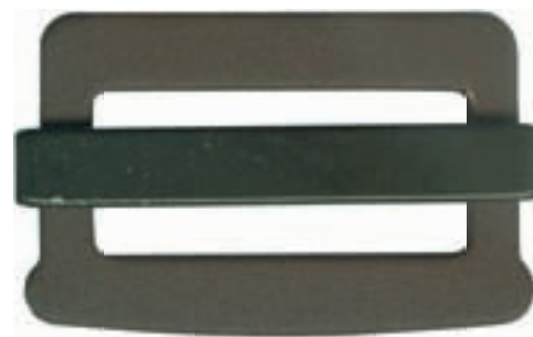
AL9 knurled adjuster bar 1 3/4" x 1" forged steel, zinc plated 5,000 lb Commercial version of PS22040 Use RH9 for certified PS22040 version.
